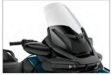
ADJUSTABLE ELECTRIC WINDSHIELD The adjustable electric windshield with memory function provides superior wind protection, and the memory function automatically returns the windshield to the lowest or previous hight.
