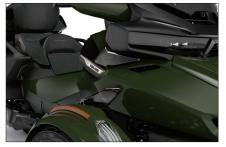
ADJUSTABLE SIDE WIND DEFLECTORS Regulate driver and passenger lower-body airflow. Change to closed, open or parallel position for optimal comfort. Simple, tool-free adjustment so you can spend more time riding.
